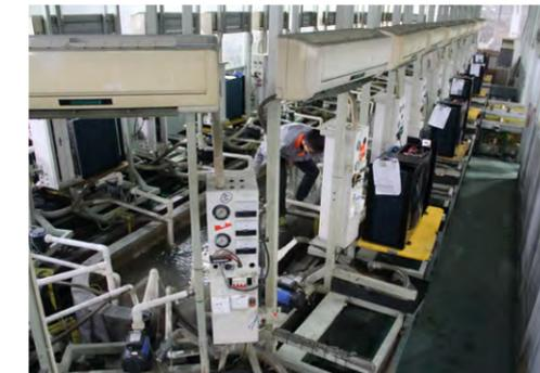
2 times leakage test of Titanium heat exchanger
